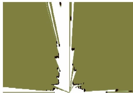
Fig. 4. Occupancy grid obtained from a laser range-finder.
