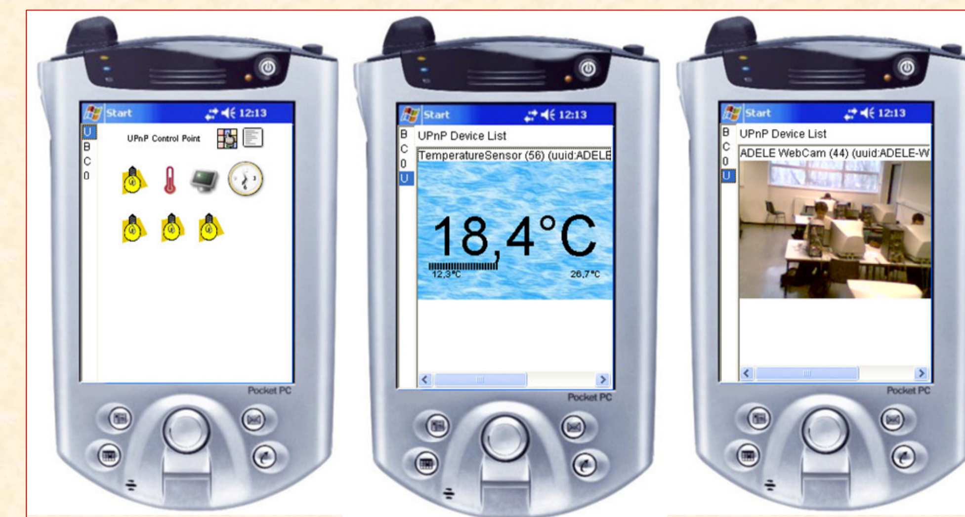
Figure 2. Controlets for a PDA-based generic control point
