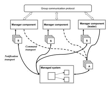
Figure 2. Replication structure
