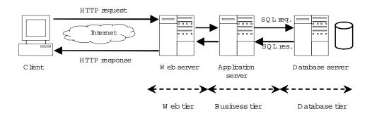
Figure 3. Architecture of J2EE applications
